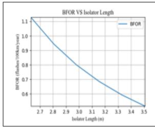
Figure 18. Effect of length of the insulator on the BFOR value
