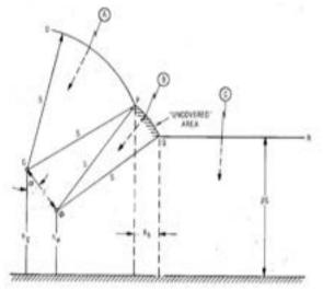
Figure 7. Simple concept of unshield area with electrogemetric theory
