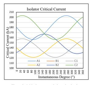
Figure 8. Critical current and phase domination Where  $\boldsymbol{\theta}_1 \, \text{dan} \, \boldsymbol{\theta}_2$  is instantaneous degrees domination in radiant. To determine critical current probability that exceeds  $\vec{I}_{cn}$  can be computed using Equation 5. 3) Compute BFOR
