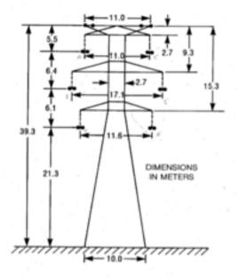
Figure 9. 345 kV transmission tower configuration
