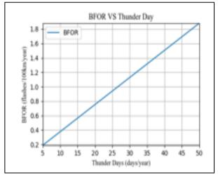
Figure 14. Effect of thunder day variations on BFOR, with feet tower resistance 20  $\Omega$
