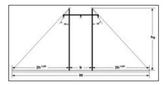
Fig. 3. Tower shadow width, with 3 horizontal conductor and 2 shielded wires
