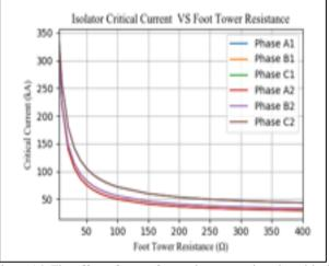
Figure 16. The effect of tower foot resistance against the critical current of the insulator, with thunder days 30 days / year
