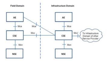
Fig. 6. Functional Architecture of oneM2M Layered Model [24]
