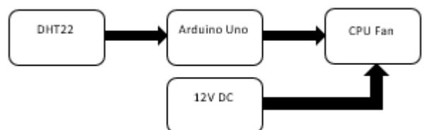
Fig.2. Block diagram
